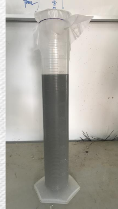
Initial Expansion and Shrinkage (ASTM C827 - 82) Bleeding of Concrete (ASTM C232-71)
