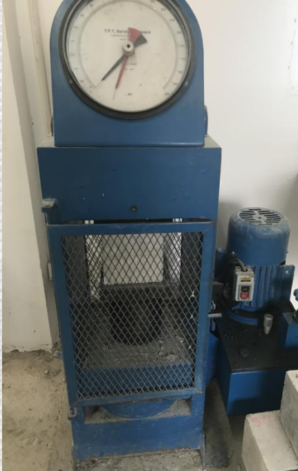
Compressive Strength of cement grout mortar (ASTM C109)
